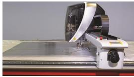
Lectra's R&D teams devoted three years to developing the technology required for zero-buffer cutting. Improvements in hardware components, an updated equipment pilot with a powerful new algorithm, and a specially designed blade will enable automotive suppliers to achieve hundreds of thousands of dollars in material savings annually as compared to other solutions available on the market.
